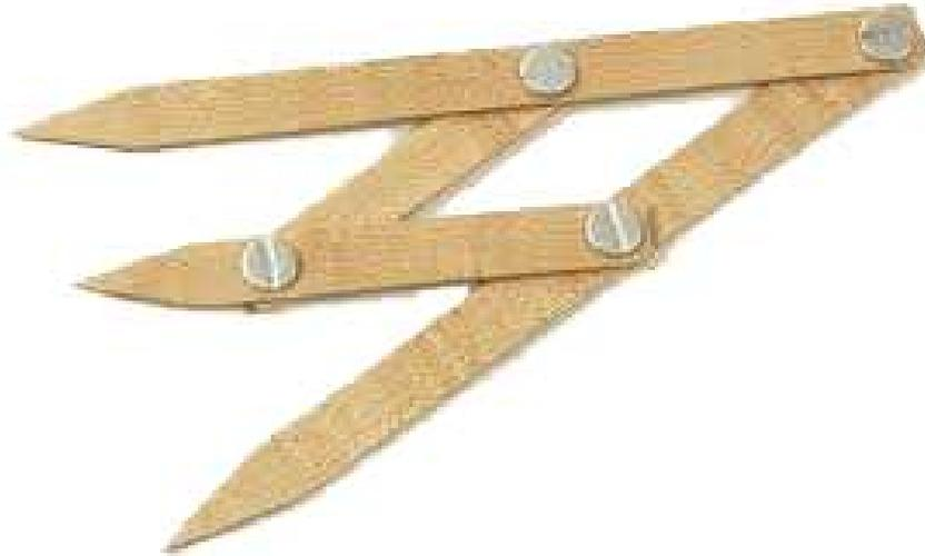
A Fibonacci Calipers is a tool for measuring the golden ratio. As you spread the two exterior legs, the middle leg will move accordingly, maintaining the golden ratio in the distances between the three legs. The golden ratio can be found in the bones in your fingers, as shown below.
